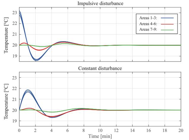
Fig. 4. Temperature regulation for impulsive and constant disturbances.
