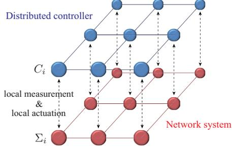
Fig. 2. Schematic depiction of distributed control systems.
