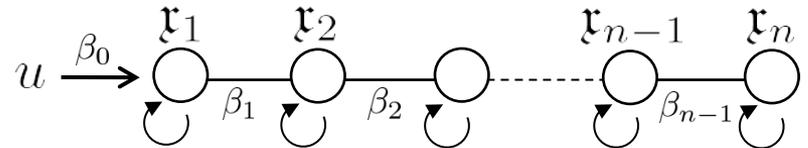
$$\mathfrak{A} = \begin{bmatrix} \alpha_1 & \beta_1 & & & & \\ \beta_1 & \alpha_2 & \beta_2 & & & \\ & \ddots & \ddots & \ddots & & \\ & & \ddots & \ddots & \beta_{n-1} & \\ & & & \beta_{n-1} & \alpha_n & \end{bmatrix} \quad \text{tri-diagonal} \quad \mathbf{b} = \begin{bmatrix} \beta_0 \\ 0 \\ 0 \\ \vdots \\ 0 \end{bmatrix}$$
