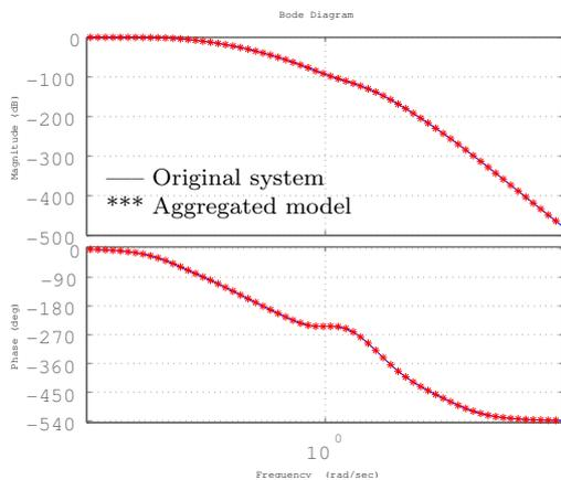
Fig. 9. Bode diagrams of original system and aggregated model
