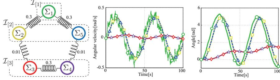
Fig. 1. Illustrative example: Networked oscillators model having five subsystems and their input responses. Angular velocities (in the middle figure) and angles (in the rightmost figure) of individual subsystems are depicted by the lines with markers  $\circ$ ,  $\square$ ,  $\diamond$ ,  $\star$  and  $\triangle$  for  $i$  in the ascending order.
