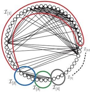
Fig. 2. Network structure of the IEEE 118 test system and resultant cluster sets for  $L = 12$ .
